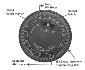
When setting the programing tabs of the timer, set the pump to operate around your peak use times. (I.e. 30 minutes before the first shower until 15 minutes after last shower).
